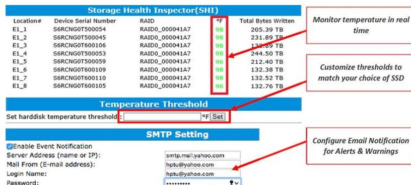
SHI (Storage Health Inspector) enables administrators to monitor the temperature of each NVMe SSD in real time, and configure warning thresholds to correspond with each make & model, via the WebGUI and CLI software suites.
