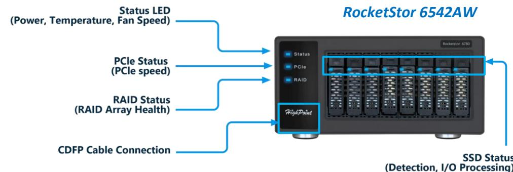
These integrated, self-diagnostic and monitoring services actively survey and report the status of the CDFP connection, PCIe lane assignment of the adapter, enclosure / SSD temperature, and the condition / status of SSDs & RAID arrays. Each service works in conjunction with the WebGUI & CLI software management suites.
