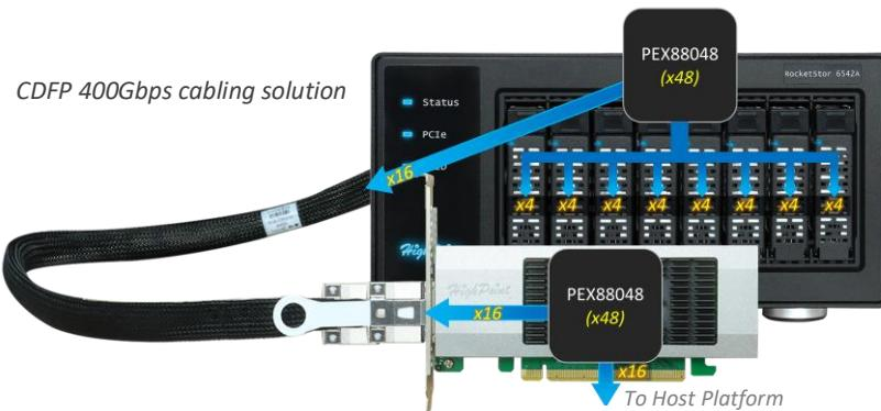
Integrated PCIe switching technology and 400Gbps CDFP connectivity enables RocketStor 654x enclosures to maximize data transfer speed by fully utilizing all x16 lanes of PCIe bandwidth provided by the host platform. Both the enclosure (device-side) and PCIe adapter (host-side), are equipped with dedicated PCIe switch ICs. This enables each solution to provide x16 lanes of dedicated PCIe Gen4 upstream bandwidth and x4 lanes of dedicated downstream bandwidth to each U.2 or U.3 SSD.
