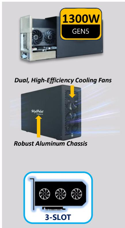
**Massive 1300-Watt PSU:** The RocketStor 8631D upscales power support from 850W to 1300 Watts via a new integrated PSU. This immense capacity significantly widens the range of supported compute and accelerator cards from all vertical industry applications. It guarantees dedicated, stable power delivery for performance-hungry workflows, preventing unexpected system shutdowns and prolonging component lifespan.
