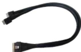
SFF-8654 (host) to SFF-8611 Oculink (device) PCIe 4.0 x8 NVMe cable. Each cable can host up to 2x NVMe SSDs.
