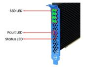
A built-in LED notification system enables administrators to instantly assess the current status, temperature and host connectivity of the RocketAIC 7608AW and hosted NVMe storage. One Led is provided for each of the 8 device channels; these are designed to work in tandem with a dedicated Status and Fault LED – simple color coding and flashing patterns can indicate everything from the strength of the current PCIe connection to progress of a RAID rebuild session.
