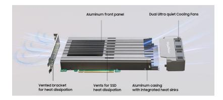
The dual-width architecture's unique socket design enables the 990 PRO SSDs to be arranged vertically, similar to how memory is installed into a conventional motherboard. This ensures each SSD is exposed to the airflow ingested by a pair of powerful, low-decibel cooling fans. Cool air is condensed and circulated throughout the casing, which then rapidly ejects waste heat via the ventilated PCIe bracket.
