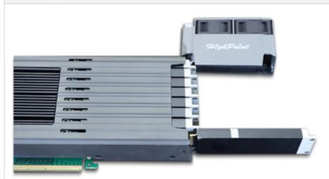
The fan-module is hinged and can be unlatched and moved counter-clockwise to expose the SSD slots.
