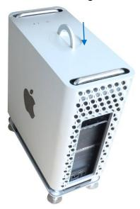
j. After the housing is fully seated, twist the top latch right and flip it down to lock it.
