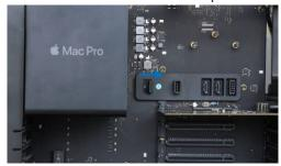
g. Using a Phillips-head screwdriver, unscrew and remove the slot cover. Remove the HighPoint NVMe RAID AIC from the PCIe slot.
