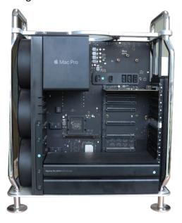
h. Reinstall the slot cover you removed, then tighten the screws on the slot cover.
