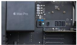
h. Install the HighPoint NVMe RAID AIC into the appropriate PCIe slot. Slide lock to locked position and install the previously removed slot cover, then tighten the screws on the slot cover.
