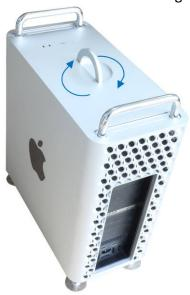
e. Lift the housing vertically upward to detach it from the 2019 Intel Mac Pro Workstation.
