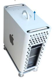
f. Slide the lock to the unlocked position.
