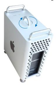
e. Lift the housing straight up and off of the 2019 Intel Mac Pro Workstation. Carefully set it aside.
