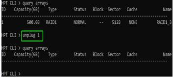
This command instructs the controller to disconnect the array "1"; you can then disconnect the drives safely.
