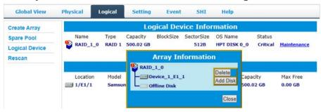
Arrays in the **Critical** status can be accessed and utilized, but are no longer fault tolerant. A Critical array should be rebuilt as soon as possible to restore redundancy.
