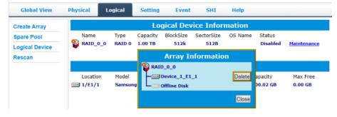
An array with the **Disabled** status means that the RAID level does not have enough disks to function.
