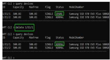
This command is used to remove the spare disk on controller 1 channel 1.
