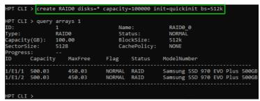
This command instructs the system to create a RAID0 array using the disks attached to controller 1 channels 1 and 2; capacity is 100GB, Block Size is 512KB.
