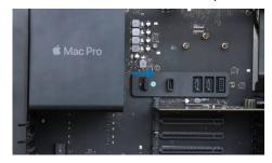
g. Using a Phillips-head screwdriver, unscrew and remove the slot cover. Remove the HighPoint NVMe RAID AIC from the PCIe slot.
