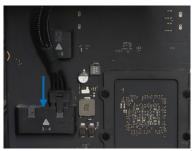
b) Connect the 6-pin power connector of the Belkin AUX Power Cable to the side of the HighPoint NVMe RAID AICs.
