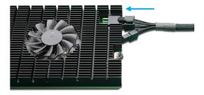
i. Install the HighPoint NVMe RAID AIC into the appropriate PCIe slot. Slide lock to locked position and install the previously removed slot cover, then tighten the screws on the slot cover.
