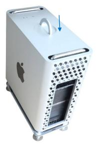
I. After the housing is fully seated, twist the top latch right and flip it down to lock it.
