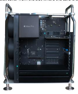
g. Slide lock to unlocked position.
