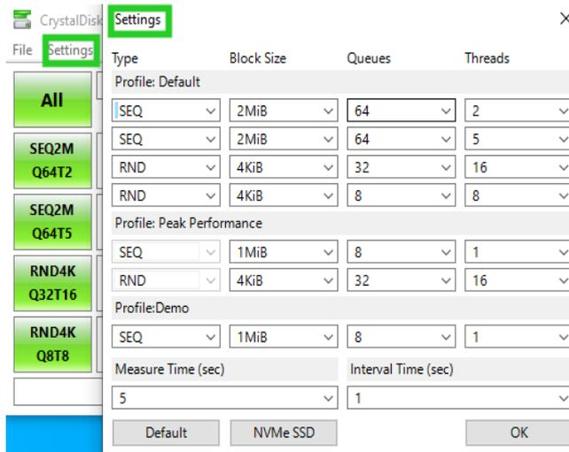
**Note2:** The above recommended setting will meet the needs of most NVMe RAID AICs and achieve optimal performance in testing. In testing, you can also choose to adjust the settings in the script yourself for optimal performance.
