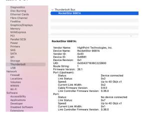
If the RocketStor 6661A entry is not displayed, this may be related to a connection problem – move the RS6661A to another Thunderbolt<sup>TM</sup> 3 port or replace the cable and recheck the entry.
