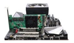
**Step 4.** Next, connect the SFF-8654 cable connector to one of the R1580B's four device ports (Ports 1 through 4)
