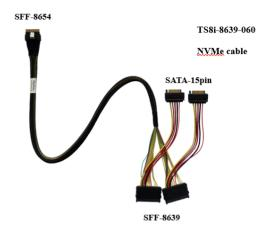
Step 2. The SFF-8654 connector should be inserted into the Rocket 1580B's device ports. The SFF-8639 connector should be connected to the U.2/U.3 SSDs (two SSDs per cable). The 15-pin SATA power cable should then be connected to the system power supply.
