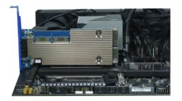
Note: Replace the full-height bracket on the R1628A with the optional low-profile bracket if required by your system.
