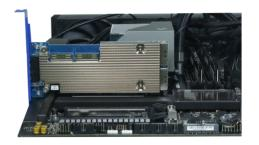
Note: Replace the full-height bracket on the R7628A with the optional low-profile bracket if required by your system.
