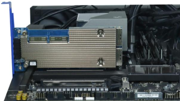
**Note:** Replace the full-height bracket on the R7628U with the optional low-profile bracket if required by your system.
