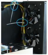
The recommended number of cable ties is between two and four, and the ties should be placed horizontally and vertically.
