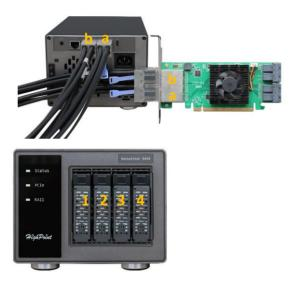
Connect the SSD6444's HBA into the PCIe 3.0/4.0 x16 slot of the motherboard;
