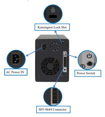
SFF-8644 Connector: SFF-8644 cable connector for HBA connection
