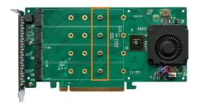
Step 4. The SSDs should be installed from top to bottom. Remove the top screw.
