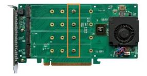
Step 4. The SSDs should be installed from top to bottom. Remove the top screw.
