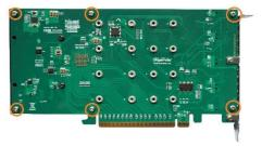
After removing the screws, carefully remove the front panel from the SSD7101A-1.
