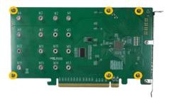
After removing the screws, carefully remove the heat sink from the SSD7104F.
