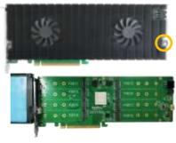
Step 3. After removing the casing, carefully turn it over to view the thermal pad. The blue films must be removed from the pad before reinstalling the panel. These films protect the pad from damage and foreign objects prior to installation, however, they will also prevent the thermal pad from conducting the heat away from the NVMe SSD's if we don't remove it.
