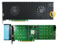
Step 3. After removing the casing, carefully turn it over to view the thermal pad. The blue films must be removed from the pad before
