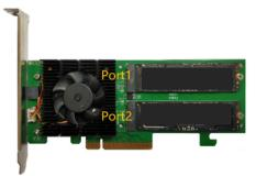
Step 7. Replace the heat sink after installing all SSDsStep 8. On the rear of the SSD7202, refasten the 4 screws that were removed in step 1.
