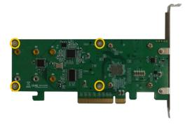
*Note:* Make sure the aluminum cover is properly aligned with the controller board (PCB), and that it makes full contact with the thermal pad, before refastening it to the SSD7202. If the cover is improperly installed, thermal pad will be unable to sufficiently cool the NVMe SSD's and controller componentry, which may result in damage to the SSD's or controller hardware, performance loss, unstable I/O, and the loss of data.
