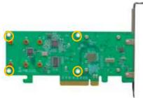
After removing the screws, carefully remove the heat sink from the SSD7202.
