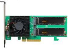
Step 7. Replace the heat sink after installing all SSDs
