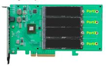
Step 7. Replace the heat sink after installing all SSDs
