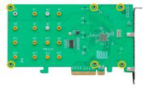
**Note:** Make sure the aluminum heatsink is properly aligned with the controller board (PCB), and that it makes full contact with the thermal pad, before refastening it to the SSD7204. If the heatsink is improperly installed, it will be unable to sufficiently cool the NVMe SSD's and controller componentry, which may result in damage to the SSD's or controller hardware, performance loss, unstable I/O, and the loss of
