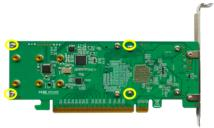
After removing the screws, carefully remove the heat sink from the SSD7502.
