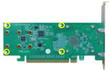
**Note:** Make sure the heatsink & fan assembly are properly aligned with the controller board (PCB), and that it makes full contact with the thermal pad, before refastening it to the SSD7502. If this assembly is improperly installed, the fan, heatsink and thermal pad will be unable to sufficiently cool the NVMe SSD's and controller componentry, which may result in damage to the SSD's or controller hardware, performance loss, unstable I/O, and the loss of data.
