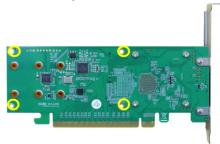
*Note:* Make sure the heatsink & fan assembly are properly aligned with the controller board (PCB), and that it makes full contact with the thermal pad, before refastening it to the SSD7502. If this assembly is improperly installed, the fan, heatsink and thermal pad will be unable to sufficiently cool the NVMe SSD's and controller componentry, which may result in damage to the SSD's or controller hardware, performance loss, unstable I/O, and the loss of data.
