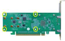
After removing the screws, carefully remove the heat sink from the SSD7502.
