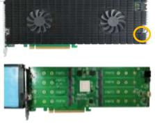
Step 3. After removing the casing, carefully turn it over to view the thermal pad. The blue films must be removed from the pad before reinstalling the panel. These films protect the pad from damage and foreign objects prior to installation, however, they will also prevent the thermal pad from conducting the heat away from the NVMe SSD's if we don't remove it.
