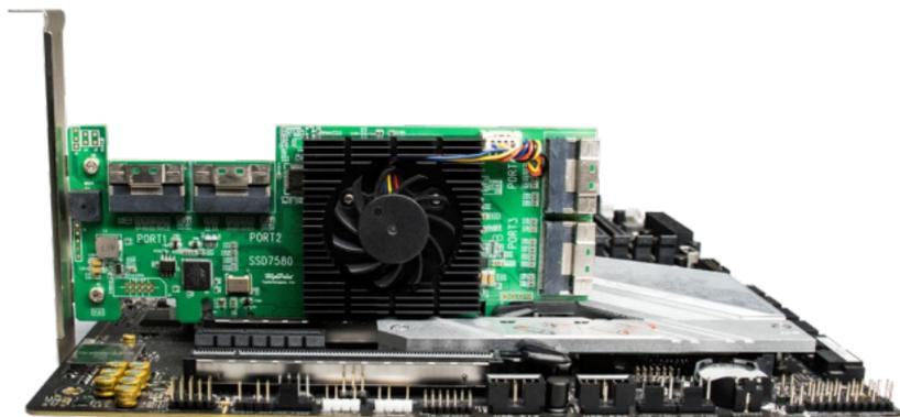
4. Connect two pieces of NVMe with SFF-8639 port, and connect SFF-8654 port to SSD7580A. Connect the 15-pin SATA power connector to the system's power supply.
