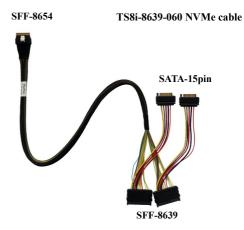
Shown above is an SFF-8654 to U.2 SFF-8639 cable with a 15-pin SATA power connector. The SFF-8639 port should be connected to the NVMe SSD's U.2 port. The 15 pin SATA power connector should be connected to the system's power supply.  Insert the SSD7580C controller into one of the motherboard's open PCI-E 3.0/ 4.0/ 5.0 x16 slots.
