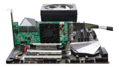
Connect the remaining NVMe SSDs to the SSD7580C controller as described above. Once complete, Power on the system.
