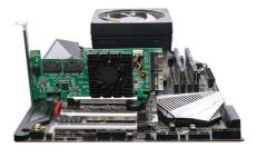
Connect two pieces of NVMe SSDs with SFF-8639 port, and connect SFF-8654 port to SSD7580C. Connect the 15-pin SATA power connector to the system's power supply.
