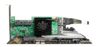
Connect the remaining NVMe SSDs to the SSD7580B controller as described above. Once complete, Power on the system.
