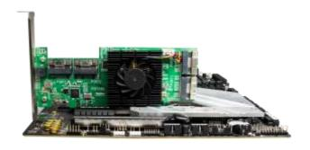
Connect two pieces of NVMe with SFF-8639 port, and connect SFF-8654 port to SSD7580B. Connect the 15-pin SATA power connector to the system's power supply.
