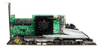
Connect two pieces of NVMe with SFF-8639 port, and connect SFF-8654 port to SSD7580B. Connect the 15-pin SATA power connector to the system's power supply.
