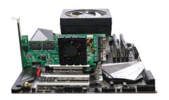
4. Connect two pieces of NVMe SSDs with SFF-8639 port, and connect SFF-8654 port to SSD7580C. Connect the 15-pin SATA power connector to the system's power supply.
