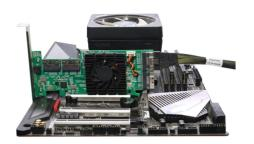
Connect the remaining NVMe SSDs to the SSD7580C controller as described above. Once complete, Power on the system.
