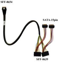
2. Shown above is an SFF-8654 to U.2 SFF-8639 cable with a 15-pin SATA power connector. The SFF-8639 port should be connected to the NVMe SSD's U.2 port. The 15 pin SATA power connector should be connected to the system's power supply.
