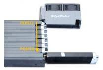
**Note:** Make sure the SSD contacts ("golden fingers") are clean prior to installation.
