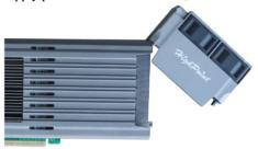
Step 2. Gently insert the SSD into the slot.
