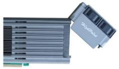
*Warning:* Please pay attention to opening the fan module carefully to avoid causing damage to the fan module
