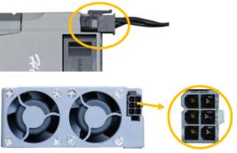
Connect 6 pin PCIe power cable
