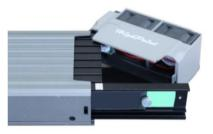
Repeat Steps 1 to 5 to install the remaining NVMe SSDs. The following example shows eight Gen4 SSDs installed into Ports 1-8:
