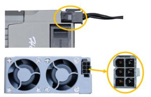
Connect 6 pin PCIe power cable
