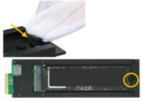
Step 8. Rotate the direction of the rubber so that it points to the left to better secure the NVMe SSD.
