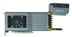
Note: Ensure the NVMe SSD Tray is carefully but securely mounted to each port. Loose connections can cause various stability and performance issues and may ultimately result in data loss.
