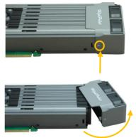
*Warning: Please pay attention to opening the fan module carefully to avoid causing damage to the fan module.*
