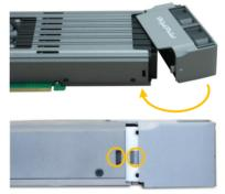
Note: Ensure the fan module is aligned correctly with the AIC board (PCB). If the fan module is improperly installed, the fan will not sufficiently cool the NVMe SSDs and AIC
